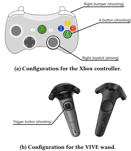
Figure 2: Xbox (top) and VIVE (bottom) controllers: On the Xbox controller, participants use either the “A button” or the “right bumper” to shoot and the “right joystick” to aim. On the VIVE controller, participants use the “trigger button” to shoot and move the wand to aim.
